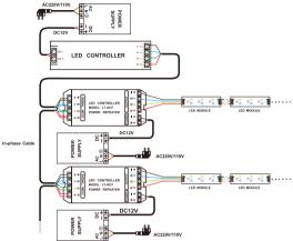
2. Repeaters Connected to DMX Constant Current Decoder:
